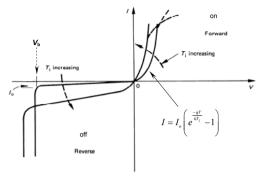
Figure 2.2. Typical I-V static characteristics of a silicon pn junction diode, and the effects of junction temperature, T<sub>i</sub>.
