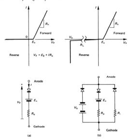
Figure 2.4. Precewise-linear approximations or junction alone characteristics:
