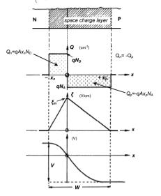
Figure 2.6. The charge Q, electric field  $\xi$ , and voltage potential V, in the space charge layer of a step pn junction.
