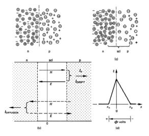
Figure 2.1. The step junction. (a) The junction if carriers did not diffuse:  $\oplus$ ionised donors. Cionised acceptors, + holes and - electrons; (b) electron and hole movements: ---- diffusion flows, —— drift flows; (c) equilibrium distribution of ionised impurities and free carriers; and (d) scl electric field and voltage.
