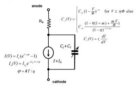
Figure 2.5. PSpice transient analysis circuit model of the pn junction diode.
