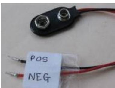
The battery snap plugs into the pins on the 5v regulator board with the red lead going to the negative output of the board as the battery snap is now DELIVERING voltage to the circuit you are powering.
