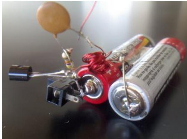
This circuit is the simplest FM circuit you can get. It has no microphone but the coil is so MICROPHONIC that it will pick up noises in the room via vibrations on a table.
