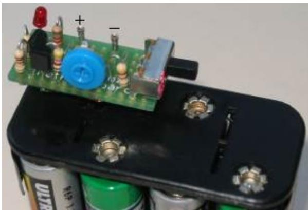
**The regulator connected to a 12v battery pack**
